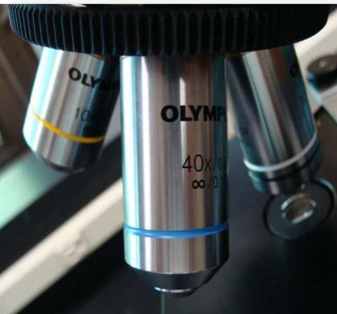
High Dry Objective Lens 40X
